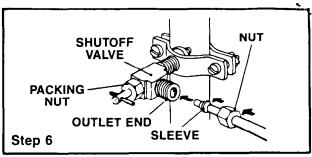
Assemble compression nuts on tubing as shown in diagram. Insert ends of tubing into connector and tighten compression nuts. Be sure ends of tubing are squarely in connector as far as they will go. Do not overtighten.
